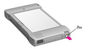
Push and release the end of the pen to take it out. You can also pull out the pen holder, just above the pen compartment, to hold your pen when it's not in use.
