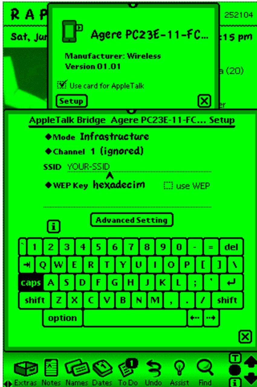
Going back to your Owner Info and the new Worksite you have created, add the 802.11b WaveLAN setup and the Internet Access settings. Once added to the Worksite, you will be able to easily edit the setup screens for your wireless adapter and add/change the WEP Keys later, if desired.
