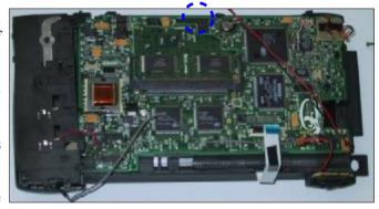
Be careful and attentious while performing this step. You have to separate the connection between the logic-board and digitizer.
